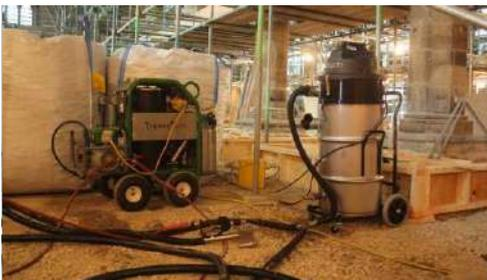
ThermaTech® and ThermaVac® systems connected together for use with internal work. The recovery head is pictured in the foreground.
