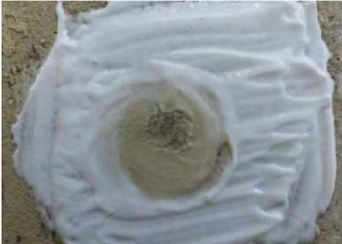
Within a few minutes a spot sample with Restorative Polyurethane Softener is beginning to mobilise after brush agitation. In this case the coating is likely to be linseed oil based but the test indicates that a combination of this softener with ThermaTech® would achieve removal. The chronology of the layering in this case indicated that the presence of lead or other heavy metal should be considered. Simple test kits for lead paint are readily available.
