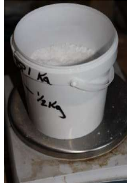
Weight/volume calibration; Ammonium Carbonate granules are weighed and the vessel marked at the corresponding volumes.
